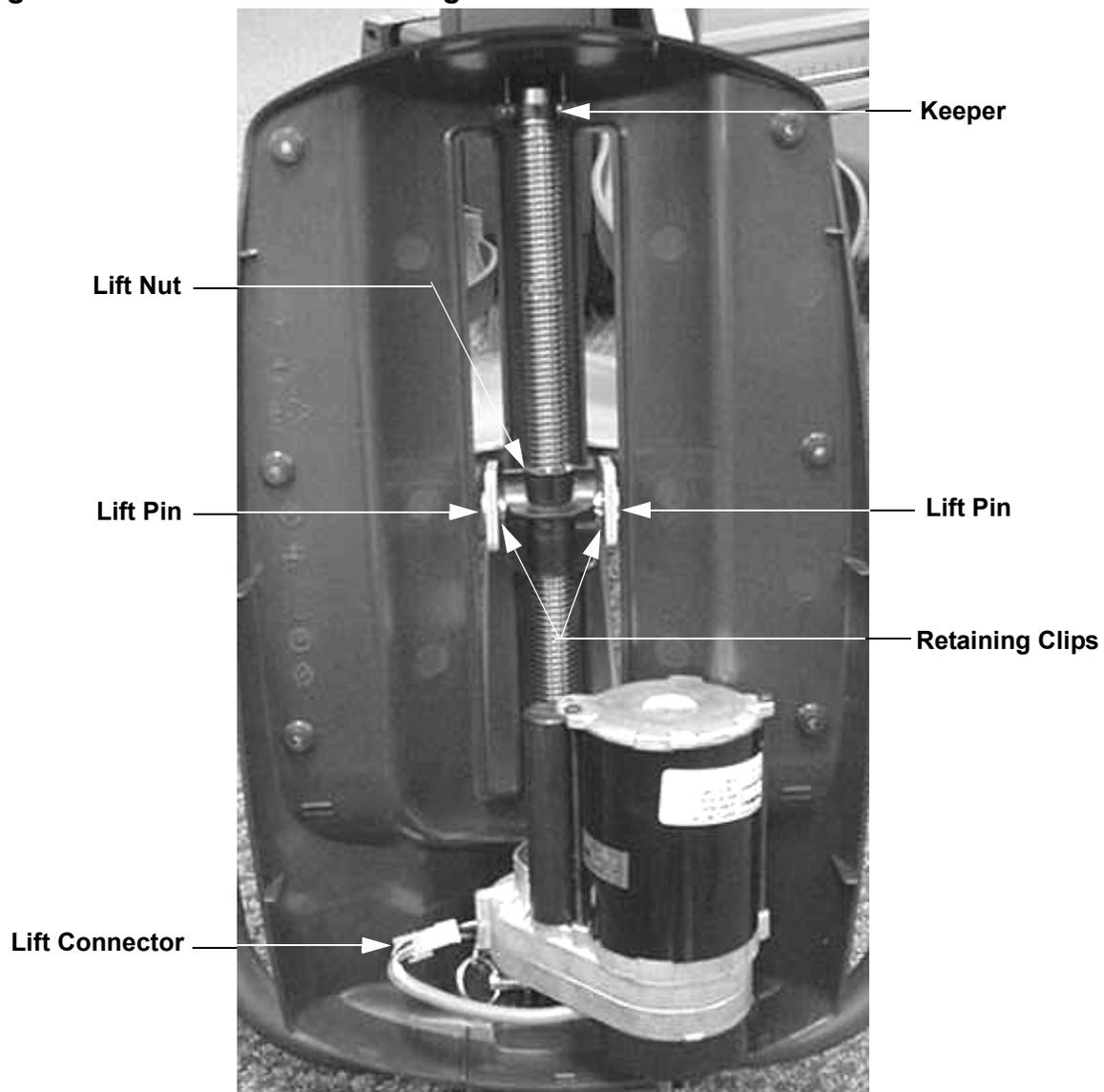
5. Remove the bolt that fastens the lower end of the lift motor to the frame. Note the location of the mylar washers, they must be replaced in the same locations to minimize lift motor operating noise.
