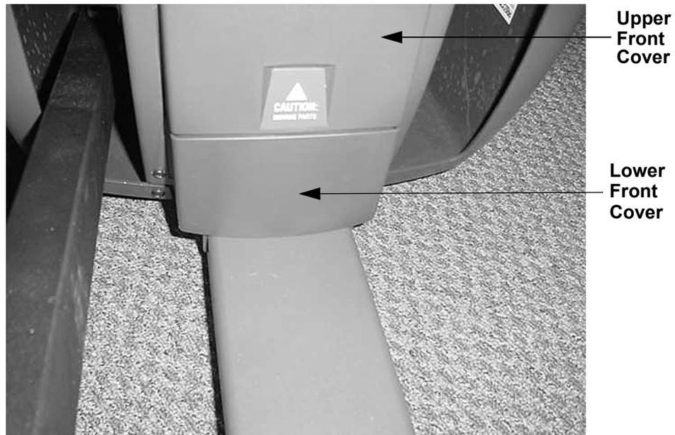
7. If all of the cover sections have been removed, first replace lower and upper front cover sections, then the top cover section and then the left and right cover sections as described below.
