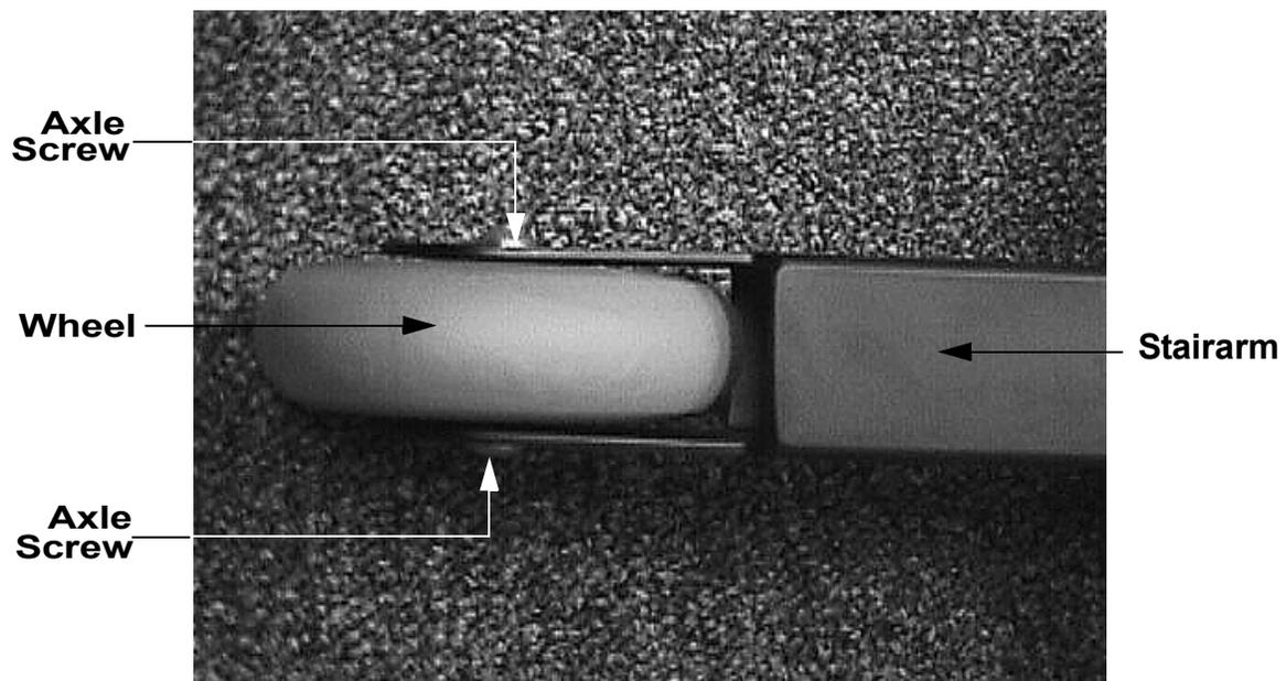
3. Set the replacement wheel in the stairarm and insert and hand tighten the wheel axle screws. Torque the wheel axle screws to 80 inch pounds.
