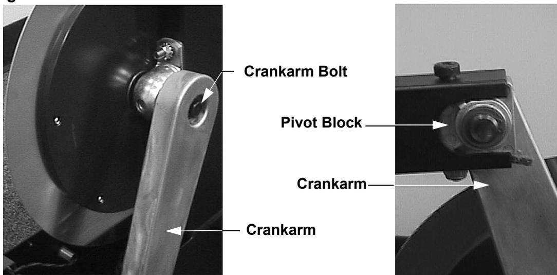
6. Clean the crankarm mounting bolt threads and the input pulley shaft threads with an alcohol swab. Allow them to dry and apply blue loctite to the crankarm mounting bolt threads.
