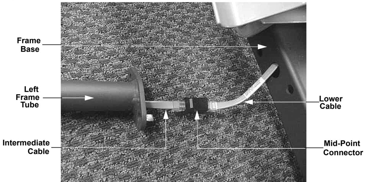
10. Disconnect the intermediate interconnect cable from the mid-point connectors at the display mounting and the lower end of the left frame tube.
