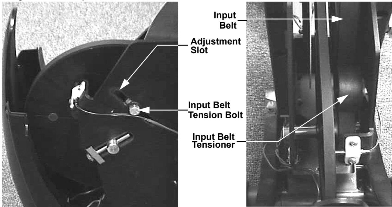
4. Loosely mount the new input belt tensioner in it's mounting position using the bolt removed in step 3.
