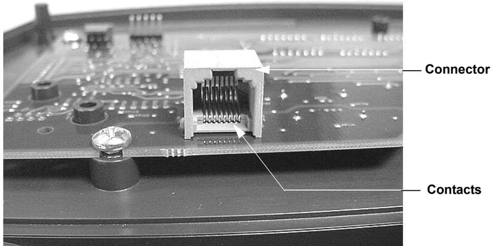
11. If the connector contacts are damaged the PCA must be replaced. Replace the lower PCA per Procedure 7.3 or the upper PCA per Procedure 7.2, as required.
