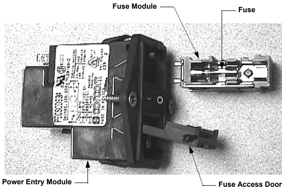
3. Using a thin bladed screwdriver, carefully pry the fuse module out of the power entry module.
