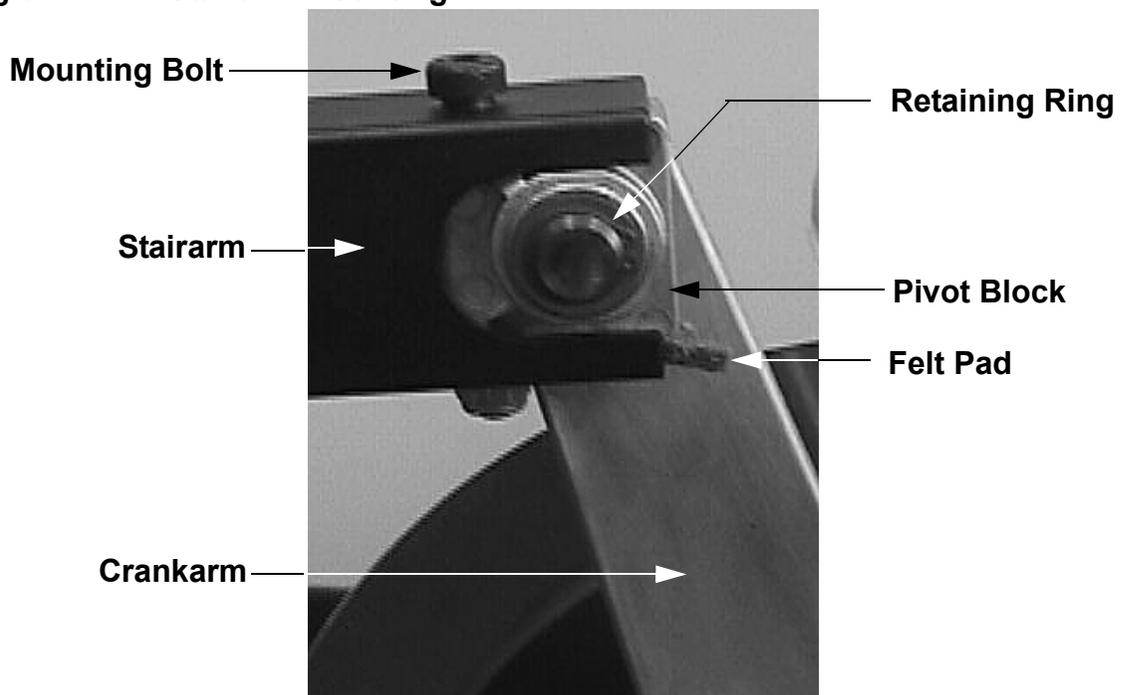
6. Slide the stairarm pivot block onto the crankarm pin and replace the retaining ring removed in step 5.
