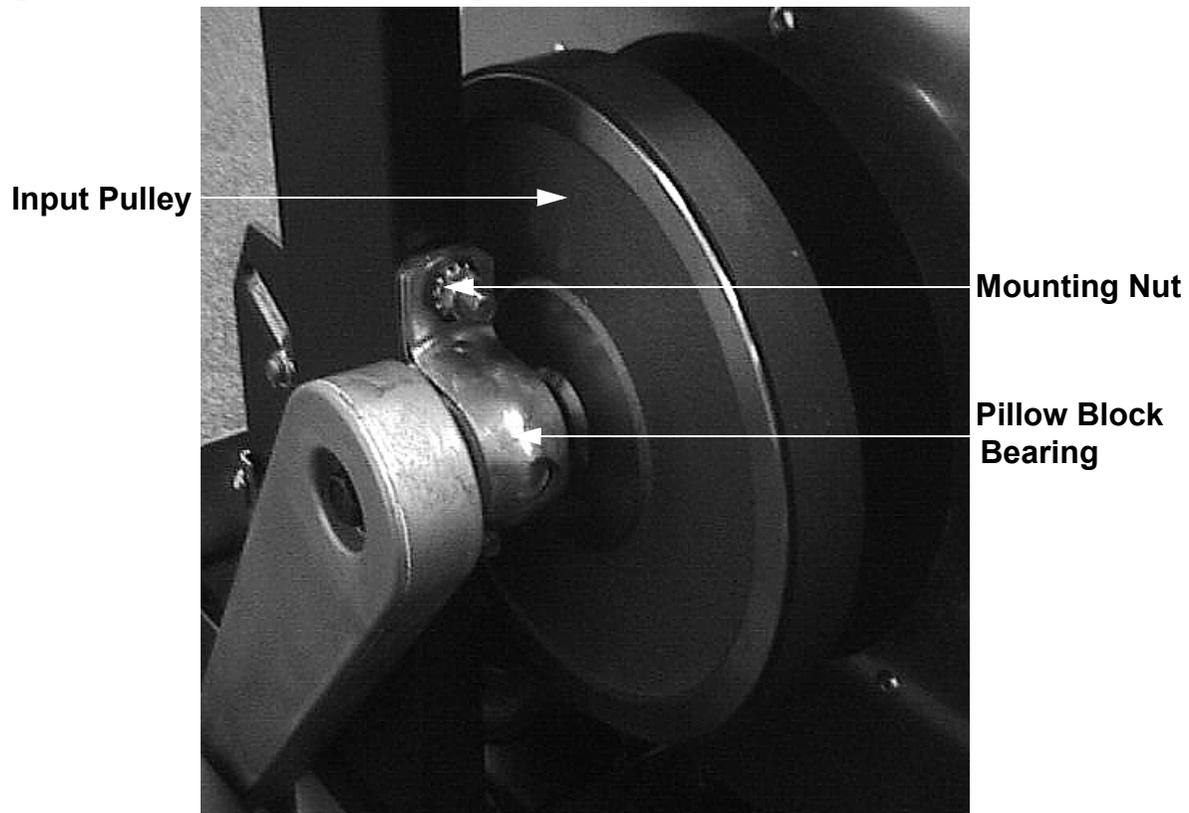
**Diagram 7.10 - Pillow Block Bearings (serial code AMPF)**
