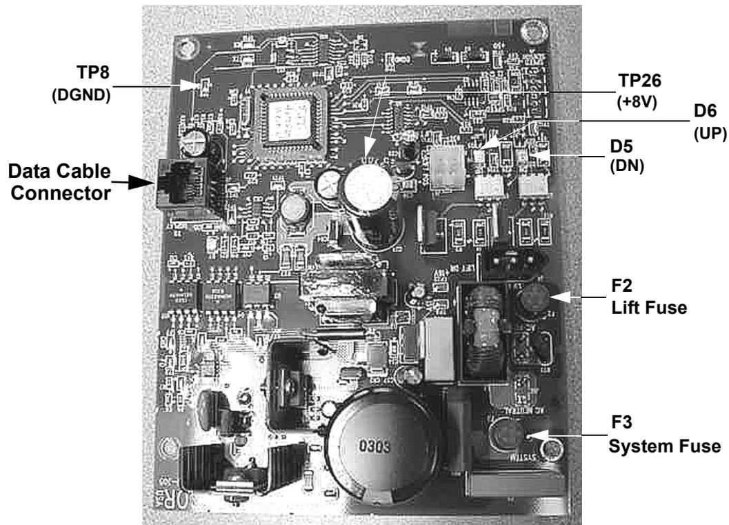
**Diagram 6.6 - Lower PCA (Serial code AMPF)**
