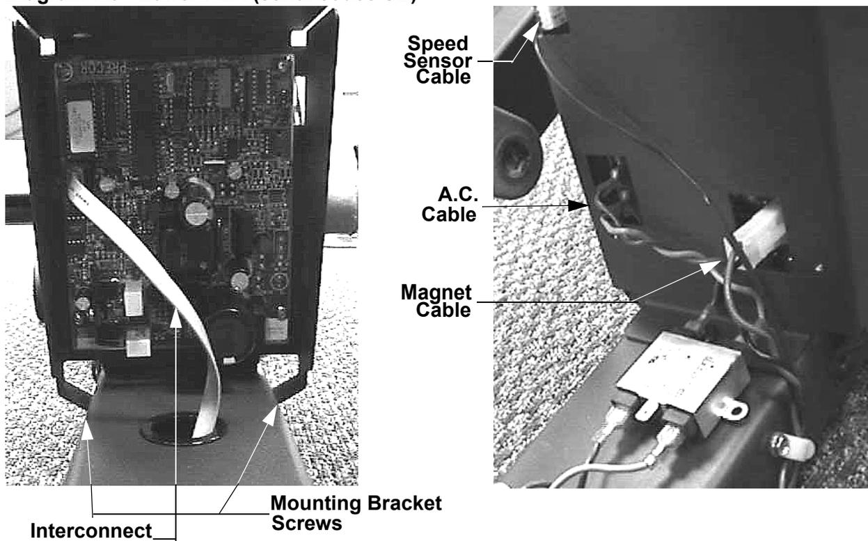
6. Carefully, rotate the lower PCA mounting bracket away from the front cover section and disconnect the interconnect cable from the lower PCA. Remove the lower PCA and mounting bracket from the unit.
