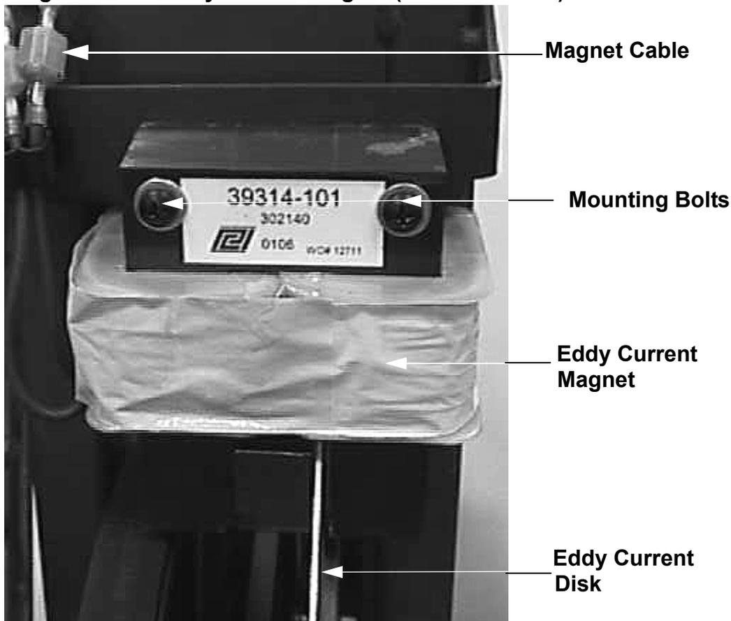
6. Position the magnet assembly at its mounting position so that the eddy current disk is centered between the magnet poles.
