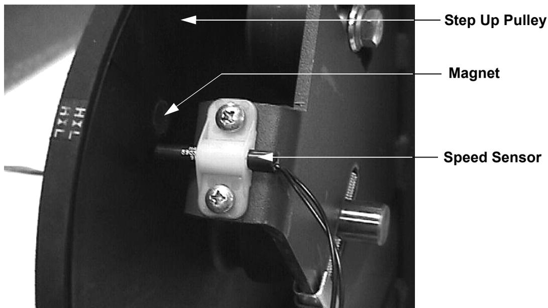
6. For serial code SB, position the speed sensor at its mounting position and set the gap between the end of the speed sensor and the step up pulley at approximately 1/8 inch. Replace the hardware that secures the speed sensor to the drive unit. Torque the speed sensor screws to 27 in./lbs.
