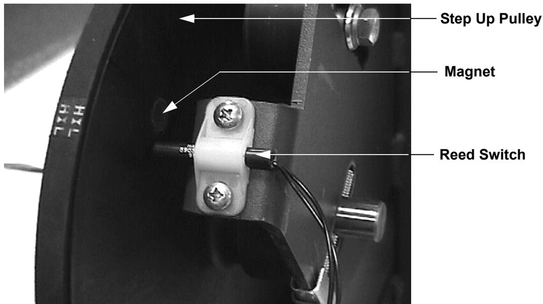
**Diagram 6.4 - Speed Sensor (serial code AMPF)**
