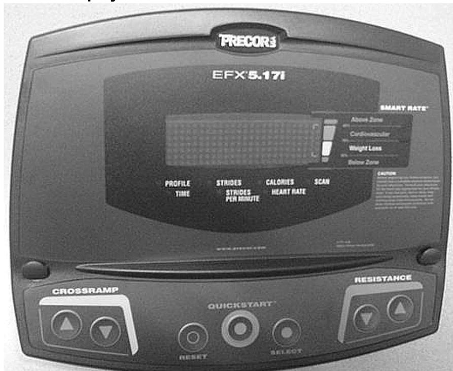
3. Watch the display as the LED test progresses. The test is programmed to display the following LED illumination sequence:
